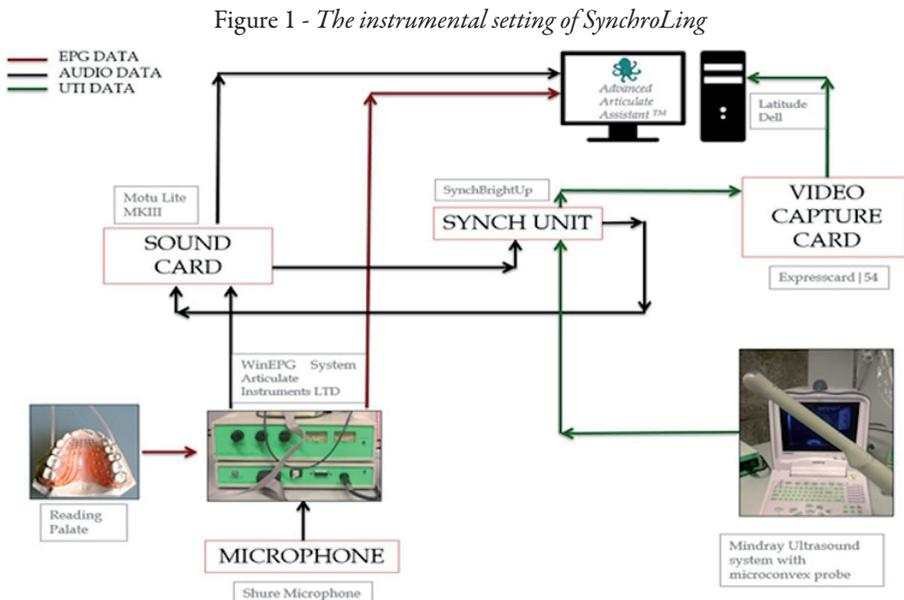
The system combines three parallel channels – one for the audio signal, one for the electropalatographic data (EPG) and one for the ultrasonographic data (UTI) (Figure 1). The EPG, UTI and audio signals were synchronized using a synchronization unit
